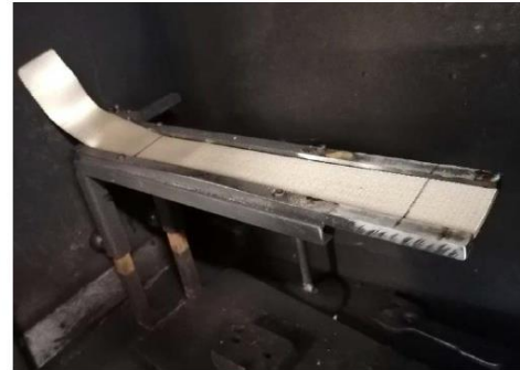
Figure 37. Seat Belt Flame Resistance, Test Set-up
