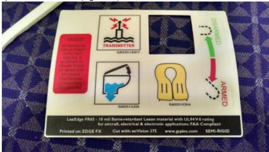
Figure 31. Colored Label Sample, After Exposure
