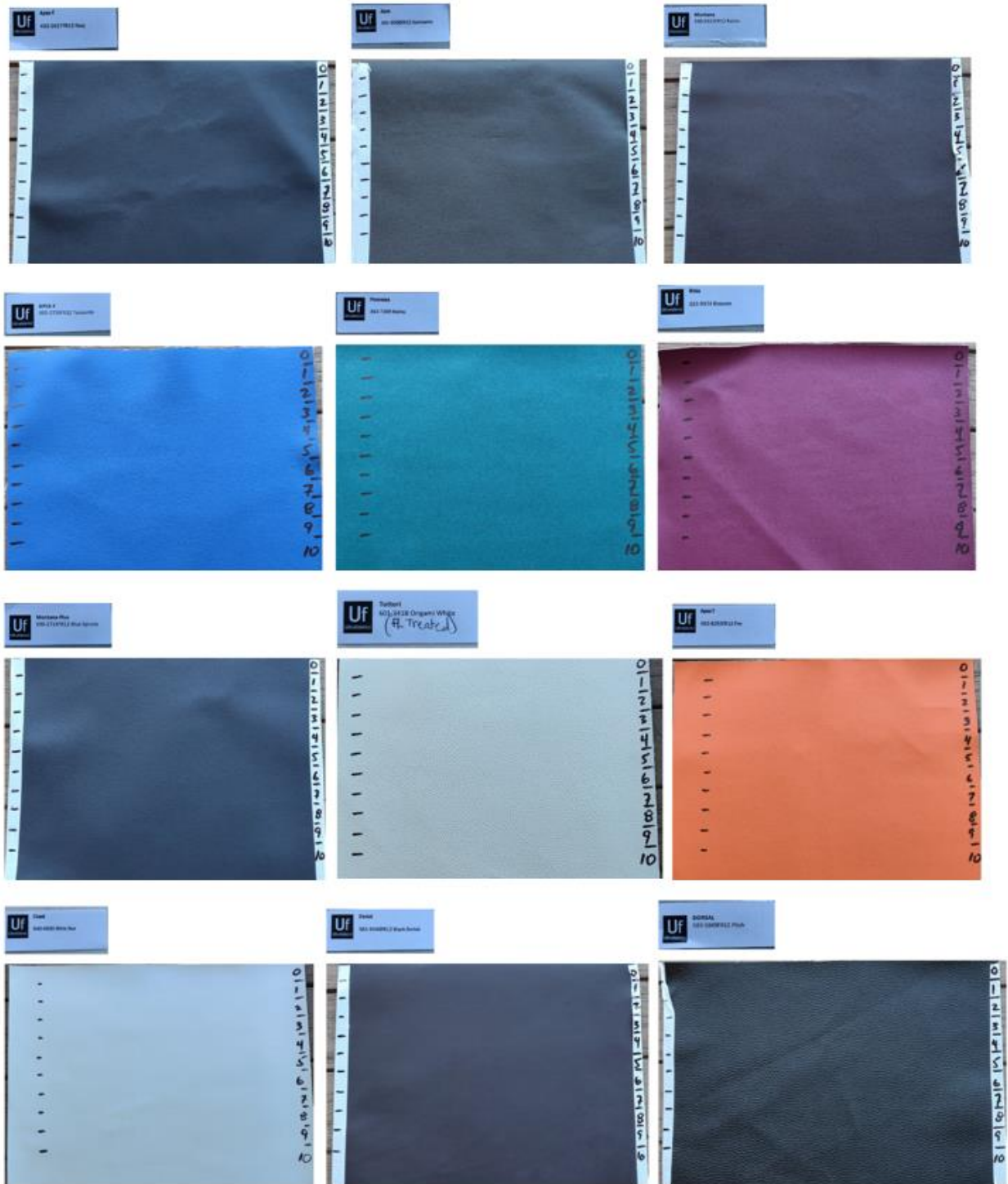
Figure 33. Ultrafabrics Samples, Progressive Exposure to 40 J/cm 2
