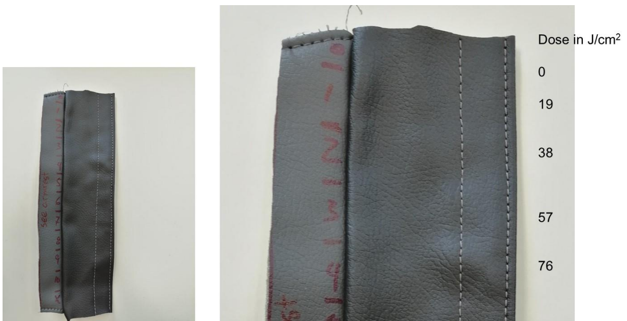
Figure 28: Leather armrest after progressive UV-C exposure. Photo on right is close up of the upper portion of the left photo, with UV-C dose marked.
